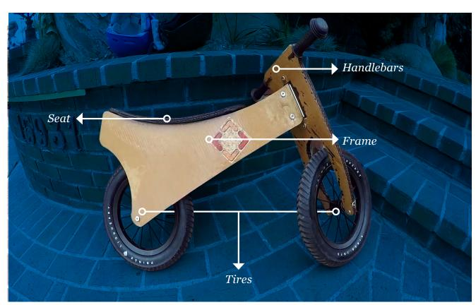
Martinez outlined the bike as having "... really only four parts. There is the seat, the frame, the handlebars/front forks and the tires." Basic hardware (nuts, bolts and rods) and strategically placed inserts hold it all together.
